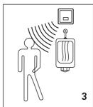
The red light will flicker every 3 seconds when the sensor detects presence. First there is a 2 seconds flush, and when the detection zone is cleared another 6 seconds flush will take place.
